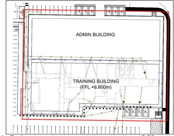
7.3.13 The 5 mm interception storage required to comply with good SuDS practice for the 2 ha Coronation Wood development area is calculated to be 100 m<sup>3</sup>. This can be adequately intercepted and captured within the infiltration systems provided for this development.
