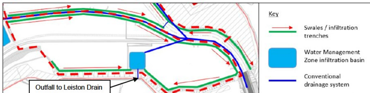
Figure 3-2 - Catchment 2 proposed drainage
