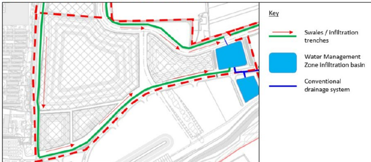
Figure 3-4 - Catchment 4 proposed drainage
