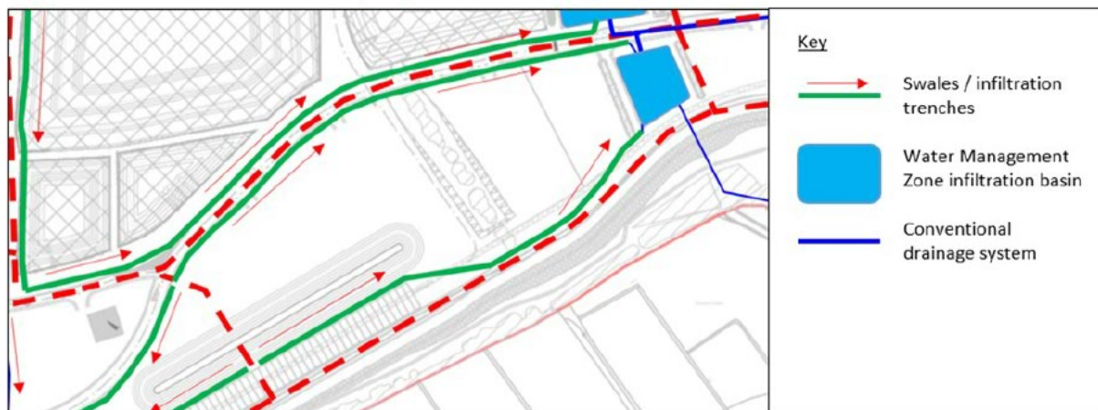
Figure 3-3 - Catchment 3 proposed drainage
