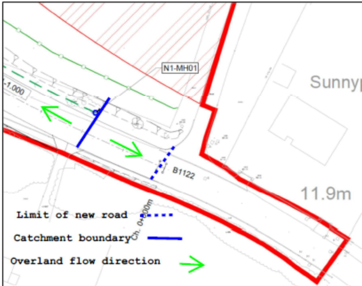
Plate 4: 20 m length of B1122 with no formal drainage
