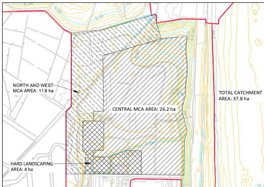
Figure 2-1 - Approximate surface water catchment area
