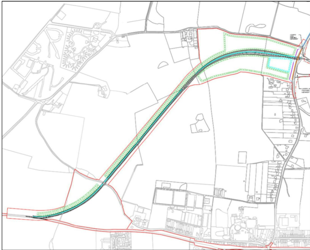
Plate 2: Green rail route from Leiston branch junction to B1122 Abbey Road showing concept drainage infrastructure
