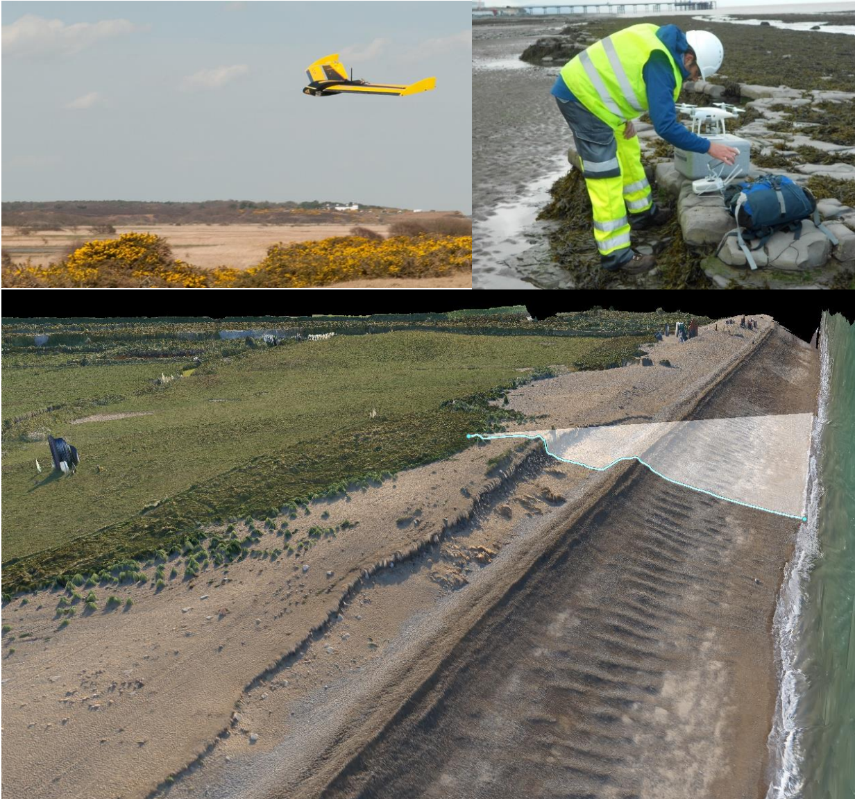
Figure 5: Fixed-wing and rotary RPA surveys at Sizewell (top left) and Hinkley Point (top right), and a Cefas RPA photo-topographic model of Cley Beach (Norfolk) viewed in perspective and illustrating the extraction of a beach profile, Norfolk (bottom).
