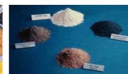
Colour can be influenced by aggregate, cement and additives, and water/cement ratio
