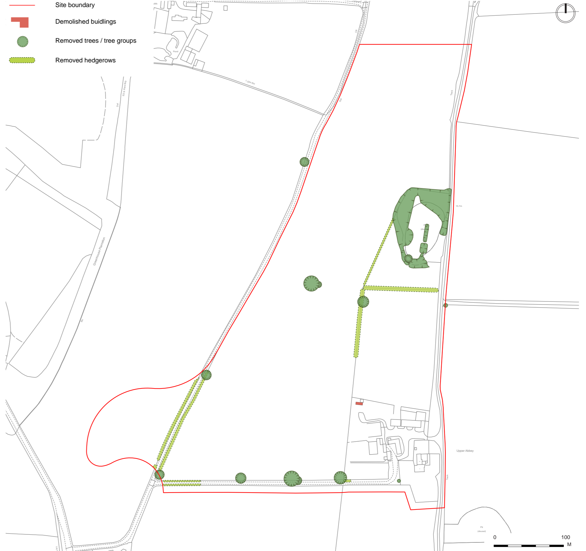
Figure A.57: Clearance and Demolition Plan
